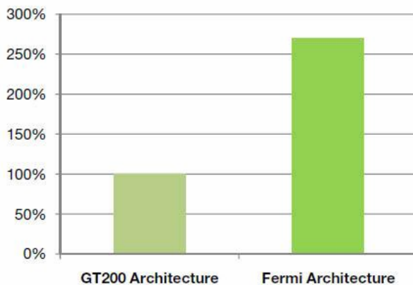
Physics algorithms such as fluid simulations especially benefit from Fermi's caches. For convex shape collisions, Fermi is 2.7x faster than GT200.
